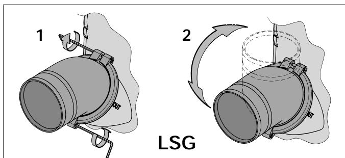
To ease the fitting of the hose to the hose connector, use only water and/or soap, NOT grease or products containing oil.
