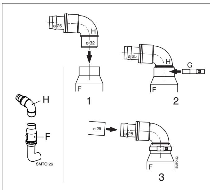
For the outlet pipe use a 25mm. internal diameter hose (such as the 'Vetus impermeable "no smell" sanitary hose'). Fix the outlet with clamps.
