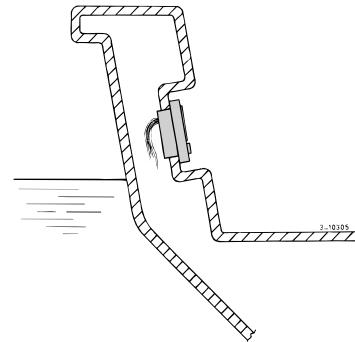
Take care that the engine panel is waterproof only on the operating side. The back of the panel should be installed in a well-protected and ventilated space. Do not install the panel where serious vibration can occur.
